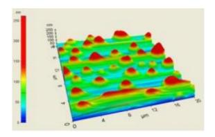
This is a non-contact atomic force microscopy showing the topography of a glass surface coated with a positively charged antimicrobial compound. Credit: The University of Manchester
