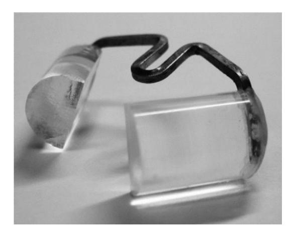
Specially designed goggles modify visual input so that only vertically oriented stimuli are perceived. Credit: Takamasa et al.
