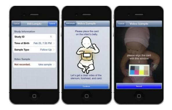
These are screenshots of the data collection app showing where to enter basic information, how to position the phone and a live feed from the camera with a view finder for aligning the color card. Credit: U of Washington
