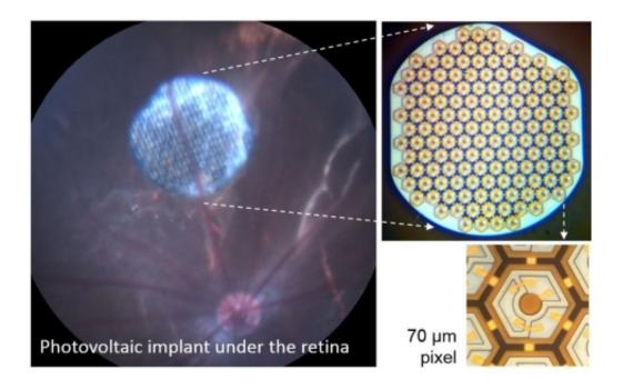
The wireless retinal implants convert light transmitted from special glasses into electrical current, which stimulates the retina's bipolar cells. Credit: Palanker lab
