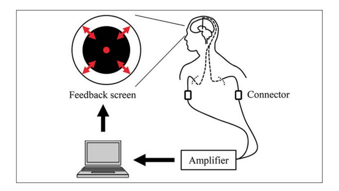
Feedback system overview. Signals from the DBS electrodes were acquired in real time. The radius of the black circle on the computer screen was controlled based on the  $\beta$ -band power of the acquired bipolar signals from adjacent contacts that were selected in the pre-feedback session. Credit: Fukuma et al., *eNeuro* (2018)
