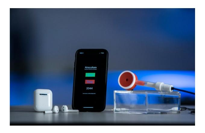
Components of the digital stethoscope developed at BYU. Credit: Nate Edwards
