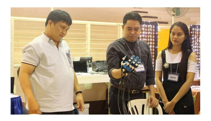
The glove of the AGAPAY Project. The robotic exoskeleton uses gamification techniques to provide patients with a high-performance treatment option in order to achieve a faster recovery rate. Credit: Agapay Project
