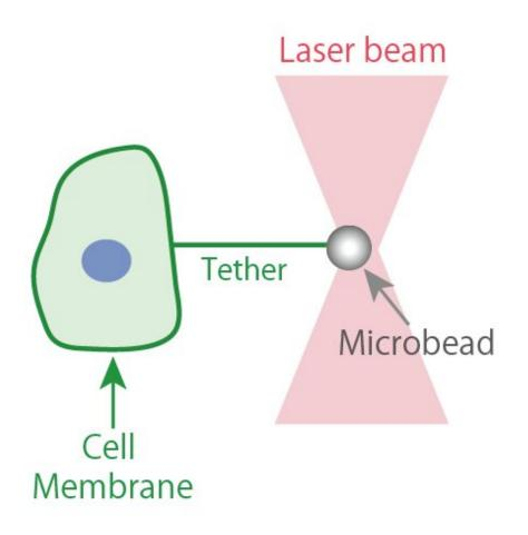
Optical tweezers are concentrated beams of laser light that can be used to trap and move microbeads. Credit: Kazuya Tsujita, Kobe University.
