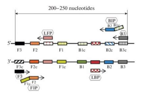
Scheme of LAMP primers: F3—forward outer primer; B3—backward outer primer; FIP—forward inner primer; BIP—backward inner primer; LFP—loop forward primer, LBP—loop backward primer. Credit: DOI: 10.1134/S0003683821080032
