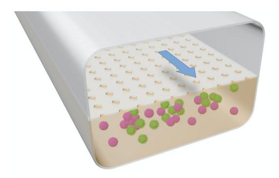
This illustration demonstrates the structure of the LF Chip: B cells and T cells were cultured together in the extracellular matrix (ECM)-lined lower channel, and were "fed" via the consistent flow of nutrient-containing medium through the upper channel. This flow is also what appears to have caused the spontaneous assembly of the cells into lymphoid follicles. Credit: Wyss Institute at Harvard University
