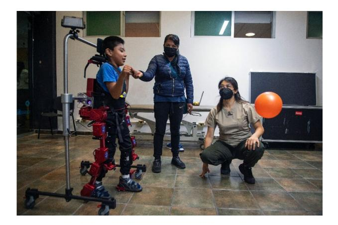
The mechanical joints of the battery-powered titanium suit adapt intelligently to the motion of each child.
