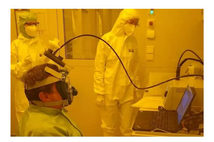
In a clean room, the particle concentration of different individuals was measured during different vocalization activities. Credit: MPI-DS / LFPB
