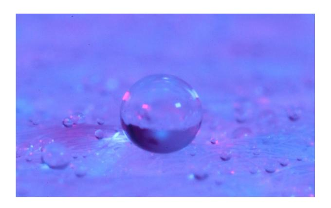
An optical image showing the water droplets in various sizes (0.2-5 mm in diameter) deposited on the fibrous surface of an N95 type mask. Credit: Sang Jin Park et al.
