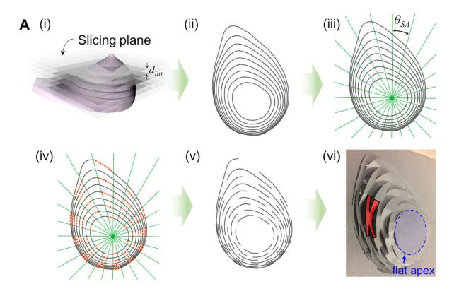
The algorithmic design process of the contour that provided topographical information of the breast. Credit: University of Pennsylvania
