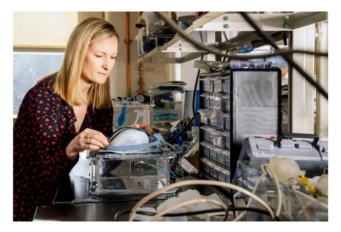
Ellen Roche and her colleagues have developed a soft, robotic, and implantable ventilator that is designed to augment the diaphragm's natural contractions. Credit: M. Scott Brauer
