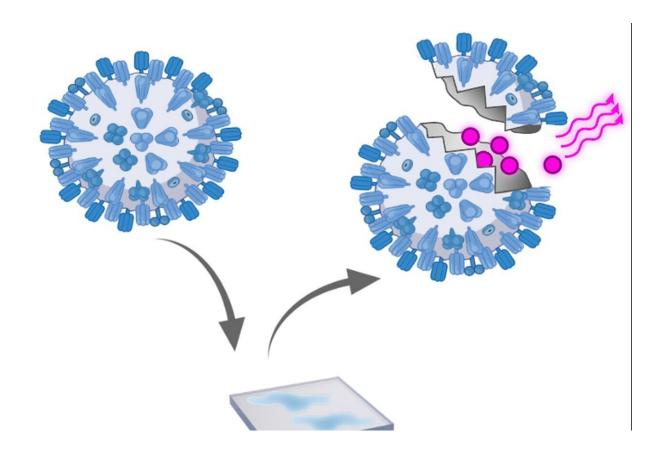
The new method is a fluorescent approach to detect viral disintegration caused by antiviral materials. Credit: Scientific Reports / Empa
