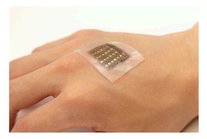
The flexible, low form-factor wearable patch comfortably attaches to the skin, allowing for noninvasive long-term monitoring of biomolecules deep beneath the skin. Credit: Xiaoxiang Gao for the Jacobs School of Engineering at UC San Diego
