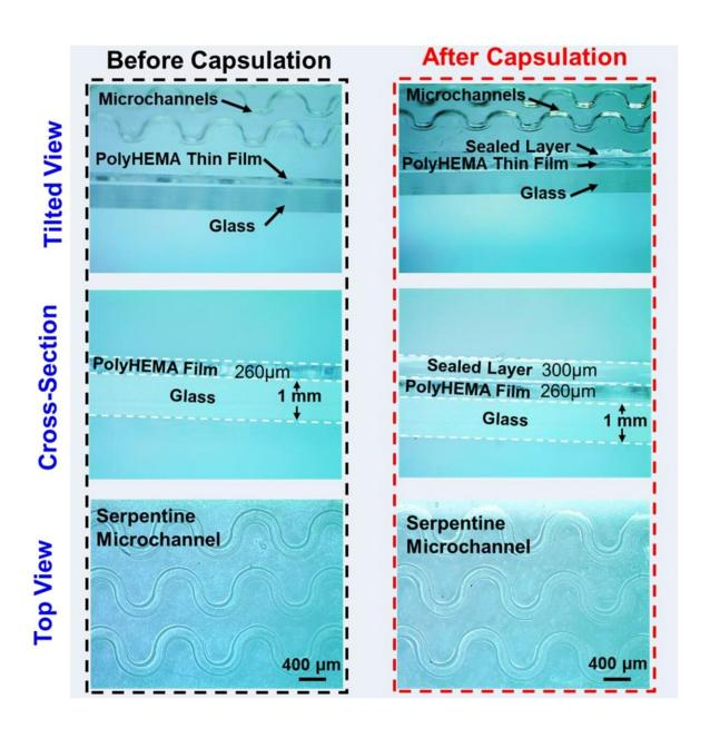
Encapsulation of the poly(HEMA) microchannels. The dimensions of
