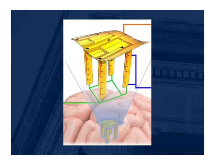
A newly developed sensor electrode device can be popped up into 3D geometry before being inserted into the brain. This design could lead to gathering more indepth information about individual neurons and their interactions with each other while limiting the potential for brain tissue damage. Credit: Huanyu "Larry" Cheng
