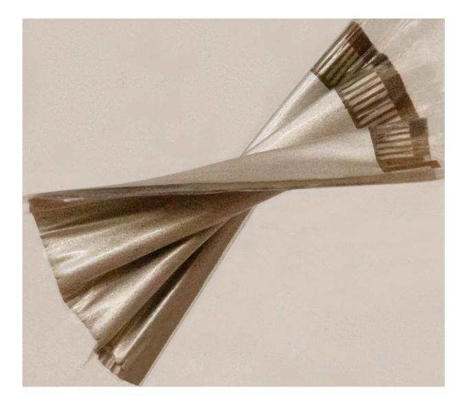
The wearable ultrasound sensor is flexible, allowing it to provide a continuous recording of cardiac activities before, during and after exercise or movement. Credit: Xu Laboratory at UC San Diego
