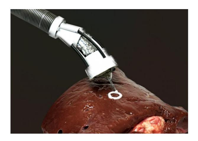
The tiny flexible 3D bioprinter developed at UNSW Sydney was able to 3D print a variety of materials with different shapes on the surface of a pig's kidney. Credit: Dr. Thanh Do
