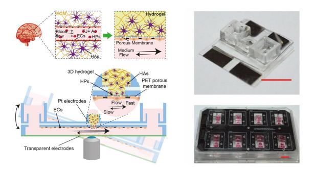
The illustration at the top left shows an in-vivo model of the blood-brain barrier, the one at the bottom left the new in-vitro model that tilts to generate liquid flow. The photos on the right show the platform on which the in-vitro model is tested. Credit: Andreas Hierlemann, Mario Modena / ETH Zurich
