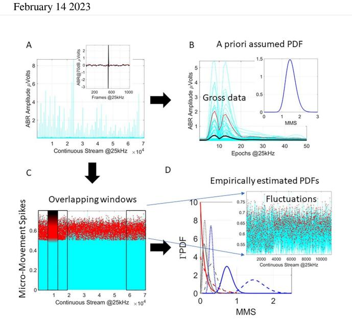
The need for new analytics. (A) Sample data from ABR pooled over multiple trials. Inset shows one trial while time series show the absolute (positively rectified) responses across trials. (B) Traditional approach is to take epochs of
