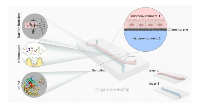
Schematic of a double layer organ-on-a-chip device. Each layer is built separately, simulating a cellular microenvironment. Credit: Valiei et al.
