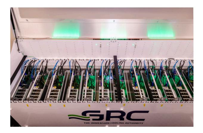
The Maverick2 supercomputer at the Texas Advanced Computing Center. Liquid immersion provides cooling for its 24 nodes of NVidia GTX 1080 Ti GPUs, with four GPUs in a node, as well as three nodes each with two NVidia P100s GPUs. Maverick2 supports GPU-accelerated machine learning and deep learning research workloads. Credit: TACC
