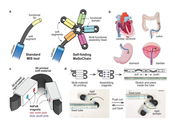
Concept and structure of magnetic soft-robotic chains (MaSoChains). a A schematic illustration of a standard MIS tool and a self-folding MaSoChain. The MaSoChains can self-fold into large assemblies at the tip of the catheter with multiple functional domains. b Potential application scenarios for MaSoChains. When pushed out of the sheathing catheter (marked in blue), MaSoChain can fold into large functional structures (colored star) in relatively open chambers in
