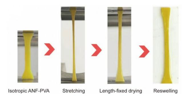
Fabrication process of the anisotropic tendon-mimetic hydrogel. Credit: The University of Hong Kong
