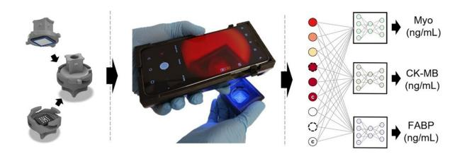
Deep Learning-Enabled Multiplexed Point-of-Care Sensor using a Paper-Based Fluorescence Vertical Flow Assay. Credit: Ozcan Lab @ UCLA
