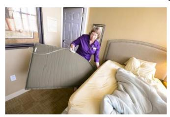
USF College of Nursing's Meredeth Rowe places one of the monitoring device's sensors beneath the mattress. The sensor detects movement and sounds an alarm to alert the caregiver if the person with Alzheimer's disease starts to get out of bed. Credit: © University of South Florida
