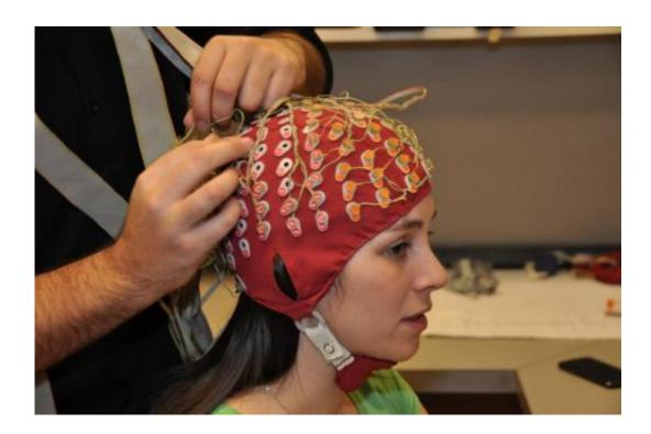
Ashley Livingstone, an SFU first year master's student, models a cap that is fitted with 128 electrodes. They are hooked up to monitor the wearer's brain activity.
