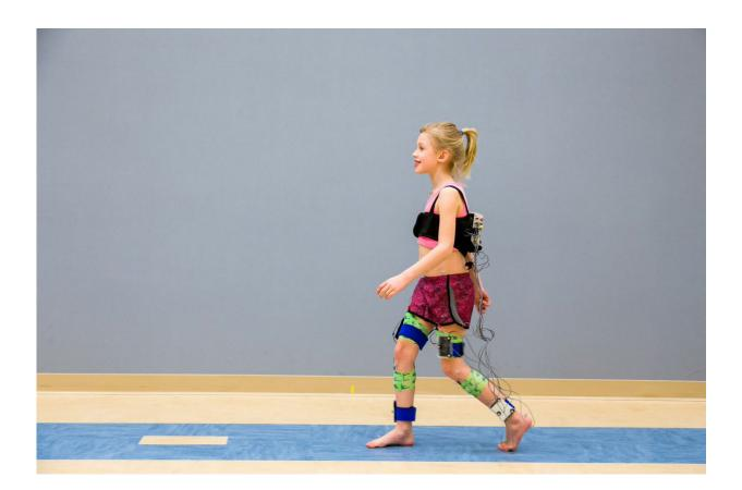
Walk-DMC is a new, quantifiable measure of motor control in children with cerebral palsy. It relies on data from electromyography (EMG) shown in this demonstration, which uses electrodes to monitor muscle activity. Credit: Michael Schwartz/Center for Gait and Motion Analysis, Gillette Children's Specialty HealthCare
