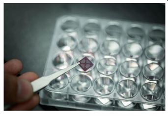
The core material used for the new immunosensor that detects proteins in the blood stream following a heart attack, providing results in just 1 minute. Credit: UNIST
