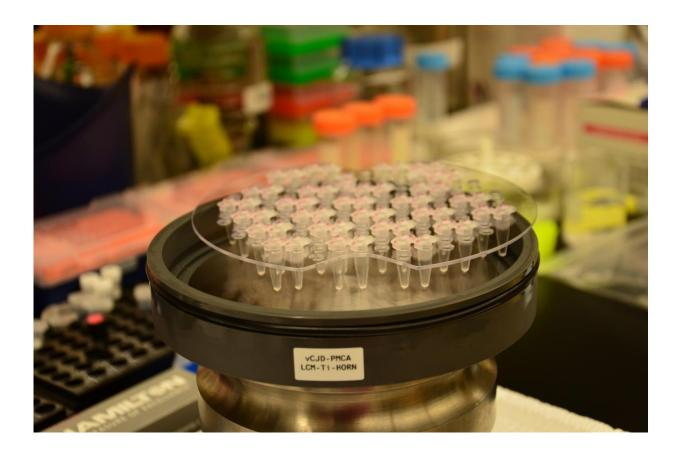
The sonicator used for Protein Misfolding Cyclic Amplification (PMCA), the amplification technique used to detect abnormal prion proteins in patient blood. Credit: Luis Concha-Marambio
