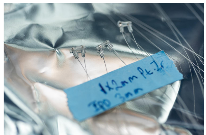
Nerve stimulating electrodes in Robert Butera's lab at Georgia Tech. Credit: Georgia Tech / Robert Butera
