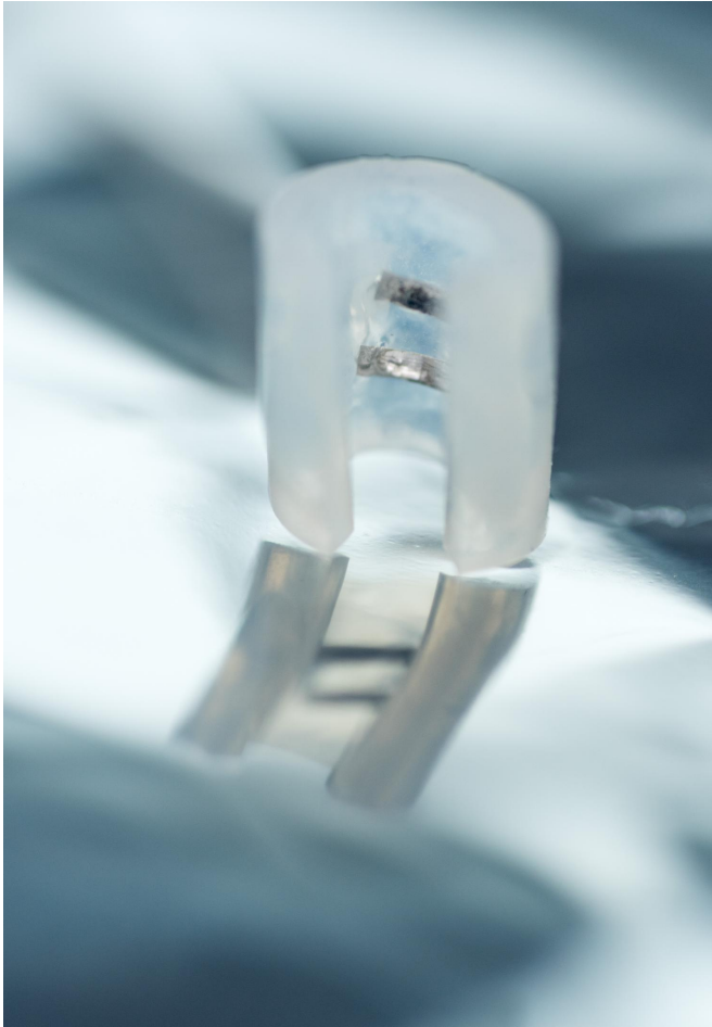
A vagus nerve implant with two contacts -- one to apply desired stimulation, the other to block unwanted stimulation. Credit: Georgia Tech / Rob Felt
