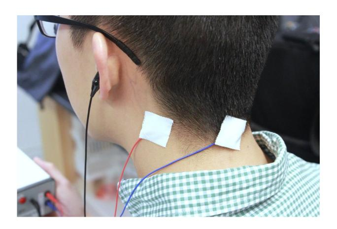
A closeup view of the skin-stimulating electrodes and earphones used to deliver the specially timed signals. Credit: University of Michigan
