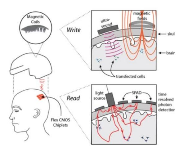
Rice's "magnetic, optical and acoustic neural access" (MOANA) device will test
