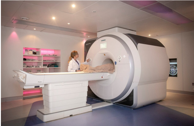
The fMRI machine located in the IDOR imaging suite. fMRI is used to indirectly detect increased neuronal activity in an area of the brain by measuring higher levels of oxygenated to deoxygenated blood. Credit: Andressa Dias Lemos, IDOR
