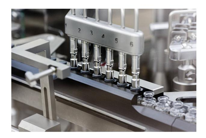
In this March 2020 photo provided by Gilead Sciences, rubber stoppers are placed onto filled vials of the investigational drug remdesivir at a Gilead manufacturing site in the United States. Given through an IV, the medication is designed to interfere with an enzyme that reproduces viral genetic material. (Gilead Sciences via AP)
