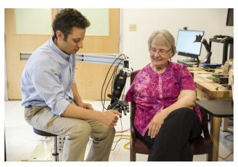
Lee Fisher, Ph.D., touches the fingers of a robotic arm, which transmits sensory information as electrical impulses delivered to the spinal cord of study participant Pat Bayne. Credit: UPMC
