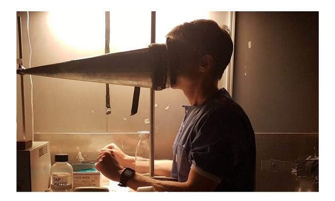
During the tests, the singers sang into a funnel. The arosol particles were measured at the other end of the funnel. Credit: Malin Alsved
