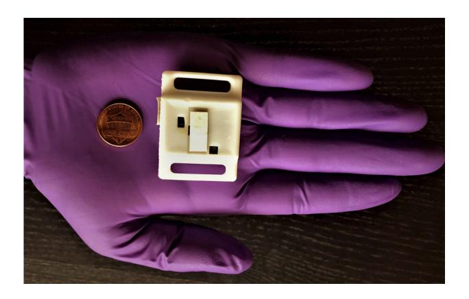
UT Dallas researchers designed a prototype of a wristwatch-like device that detects two key biomarkers associated with inflammatory bowel disease. Credit: University of Texas at Dallas
