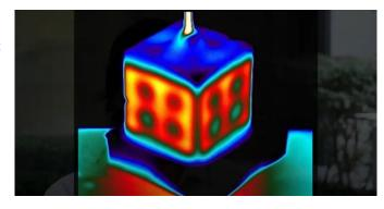
An infrared tomography of a heat-perfused hydrogel shows that, during perfusion, heat traces the path of fluid flow. In this case the spatial geometry of the channels forms a cube. Credit: Daniel Corbett
