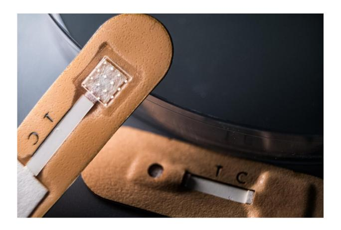
A bandagelike test for malaria features an array of microneedles that collect interstitial fluid from skin and delivers results on a test strip within minutes. Credit: Jeff Fitlow/Rice University
