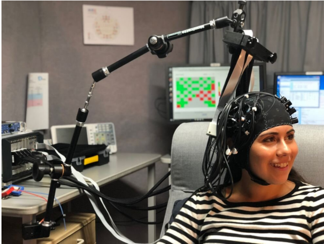
A person set up for an fNIRS recording (the brain imaging technique used in this paper). Credit: Mehrnaz Shoushtarian
