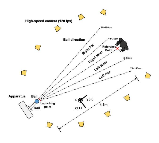
Fig. 1 Experimental set-up. Credit: University of Tsukuba
