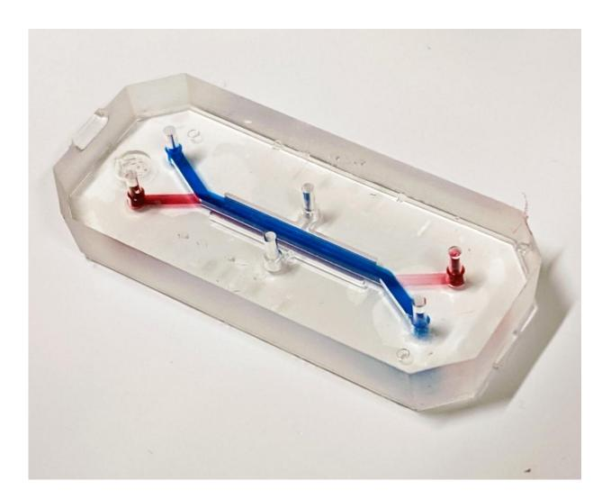
A close-up image of the lung-on-chip model used in the study. The endothelial or vascular channel is highlighted with a red food coloring dye, and the epithelial or airway channel is highlighted with a blue food coloring dye. The design allows for a co-culture of the cells from the two channels in the middle of the chip.
