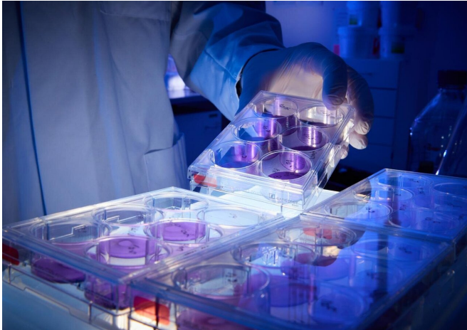
Cell culture plates with stained cells, in which virus replication can be quantified by the 'holes' that virus infection causes in the cell lawn. Credit: Volker Lannert/University of Bonn
