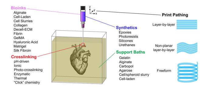
In APL Bioengineering, researchers provide perspective on the Freefrom Reversible Embedding of Suspended Hydrogels 3D bioprinting approach, which solves the issue of gravity and distortion by printing within a yield-stress support bath that holds the bioinks in place until they are cured. This image shows the customizability of the FRESH bioprinting platform. Credit: Adam Feinberg and Andrew Hudson, Carnegie Mellon University
