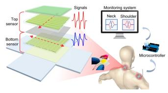
Schematic illustration of the system to prevent joint disorders. The signals produced from the attached sensors are transmitted to an intelligent terminal through a microcontroller. The multilayer sensor consists of a cross-shaped substrate, a square top sensor and a square bottom sensor. Credit: Dr. Zhengbao YANG from the City University of Hong Kong
