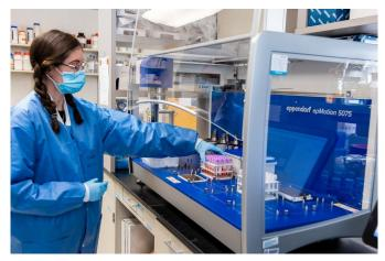
Scientists load patient sample specimens into a robotic liquid handler to prepare them for sequencing. Credit:
